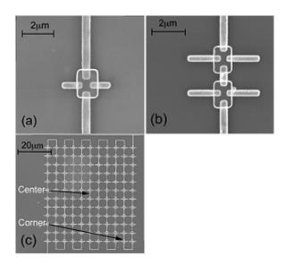
FIG. 1. SEM micrographs of the (a) single dipole nano-antenna-coupled microbolometers, (b) double dipole nano-antenna-coupled microbolometers, and (c) array of dipole nano-antenna-coupled microbolometers with annotations indicating the locations where s-SNOM measurements were performed.
