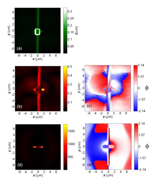
FIG. 3. Images showing simulated and measured data from the single dipole nano-antenna-coupled microbolometer structure. Shown is simultaneously recorded (a) AFM height data showing the topography of the structure, (b) measured amplitude signal from *s*-SNOM, and (c) measured phase signal from *s*-SNOM. Also shown are (d) simulated amplitude and (e) simulated phase signal calculated from COMSOL MULTIPHYSICS.
