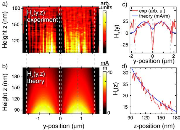
FIG. 3 (color online). Magnetic field  $H_x(y, z)$  above coupled-dipole antennas (position indicated by gray dashed lines) derived from the electric near-field distribution  $\mathbf{E}(\mathbf{r})$ , experiment (a) and theory (b). Horizontal variation of  $H_x(y)$  (c) and vertical distance dependence of  $H_x(z)$  (d) [black dashed lines in (a) and (b)]. Because of the antenna symmetry,  $H_x(y, z)$  in the  $y - z$  mirror plane represents the full magnetic antenna response.
