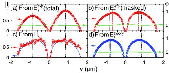
FIG. 4 (color online). Current distribution  $I(y)$  along antenna dimer reconstructed from  $E_y$  (a, total and b, masked to remove scattering due to metal roughness) and  $H_x$  (c) with normalized amplitude  $|I|$  and phase  $\phi$  [radians]. A shift in current maximum (dashed line) of 100–200 nm with respect to geometric center (dotted lines) results from capacitive gap coupling. For comparison, (d) and solid line in (c) show  $I(y)$  from theory.
