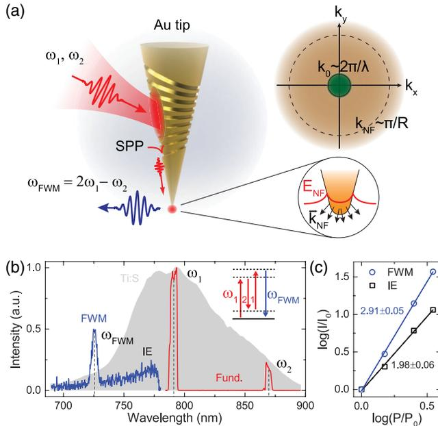
FIG. 1. (a) Experimental configuration (left), with enhanced efficiency due to the broad distribution of field momenta  $k_{x,y}$  for nanofocused SPPs associated with the gradient field and spatial confinement (right). (b) Full laser spectrum (gray), fundamental scattering off the tip apex (red), incoherent emission (IE) background, and coherent FWM peak (blue). (c) Power dependence of the FWM signal (blue) and incoherent emission (black) showing cubic and quadratic dependence, respectively.
